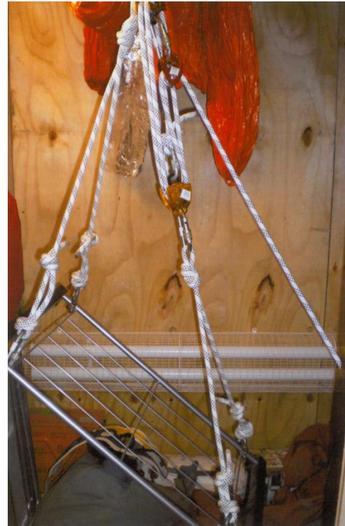
A rig for a nylon stretcher or slick (UK term) - converts from vertical to horizontal without having to rehang it.
